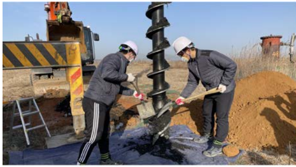
(a) Waste sampling by excavation
