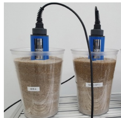
(c) TDR sensor measurement
