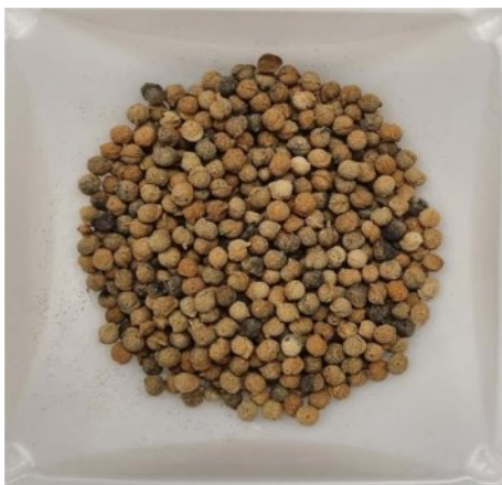
Fig. 1. Photo of alum sludge-based adsorbent (diameter: 3 mm).
