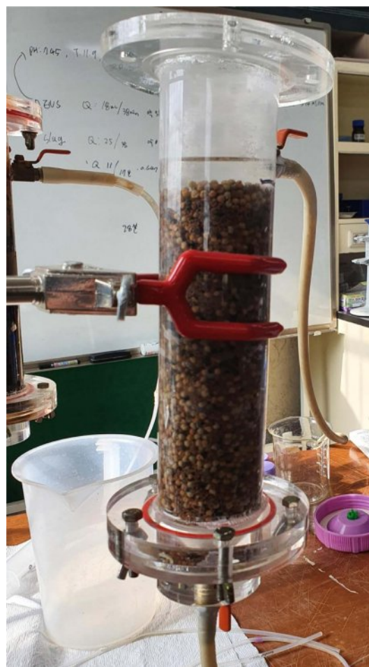
Fig. 2. Bench-scale adsorption reactor with alum sludge-based adsorbent used in this study.
