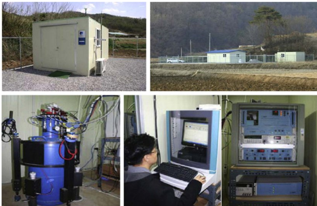
Fig. 6. Superconducting gravimeter installed and operated by Sejong University and KIGAM at the Mungyeong seismic observatory.
