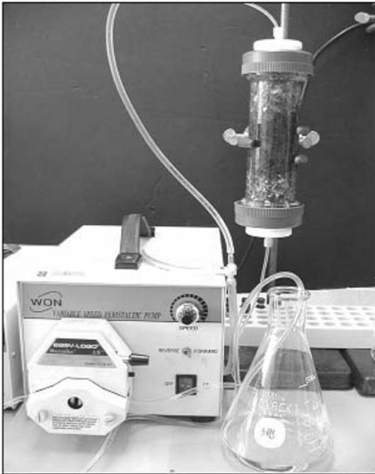
Fig. 1. Column experiment for soil washing with 20% hydrogen peroxide solution.
