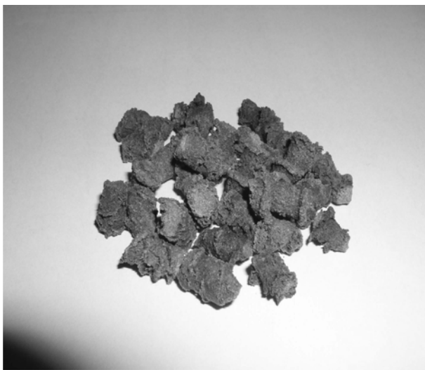
Fig. 1. Photograph of woodchip-contained plastic media (ABA-1).
