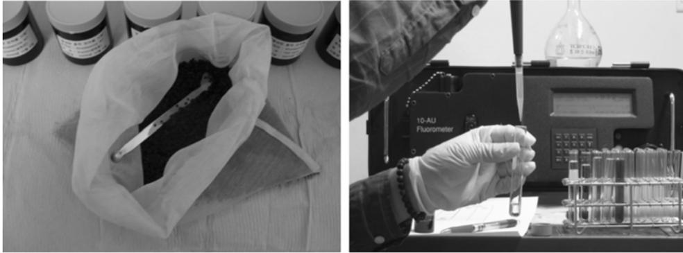
Fig. 1. Granular activated charcoal used in this study and measurement of tracer concentration using 10-AU-005-CE fluorometer.
