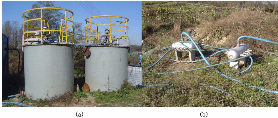
Fig. 5. surfactant storage tank & stirring system (a) and injection distributor (b).
