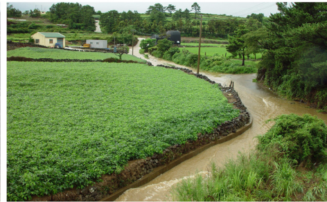
Fig. 7. The photos showing discharge of harvested rainwater from greenhouse to road without rainwater harvesting facilities resulting in flood at Hoecheon-dong.
