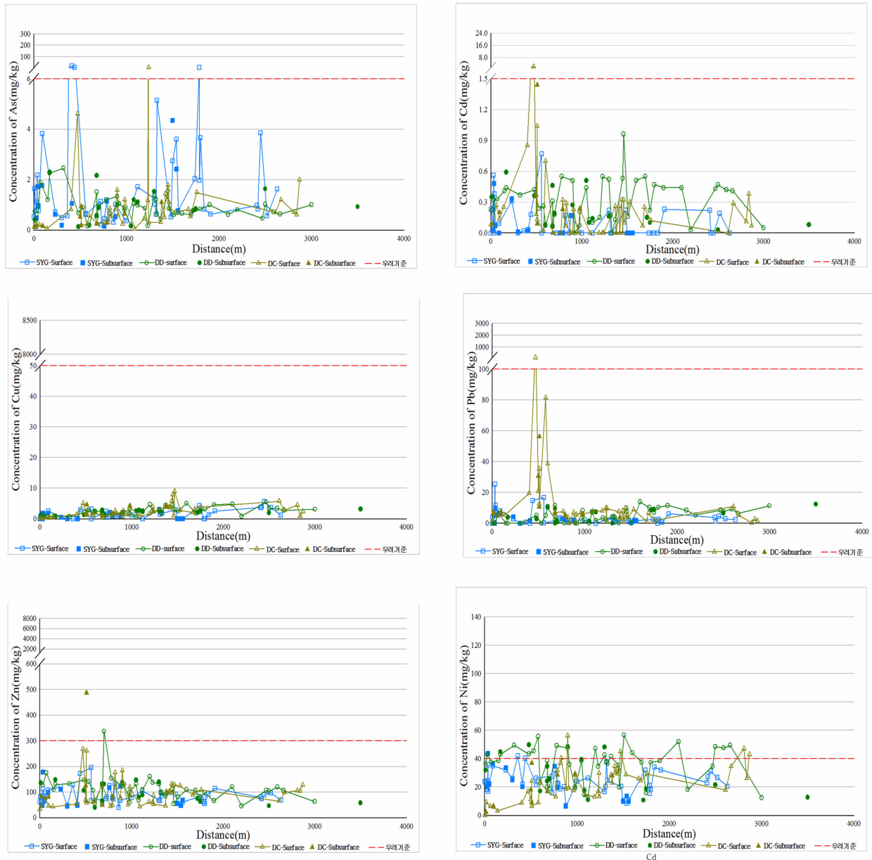
Fig. 3. Concentration of As, Cd, Cu, Pb, Zn, and Ni according to the distance from a minehead.
