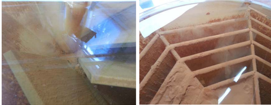
Fig. 6. Re-suspending the settled sludge in settling basins.
