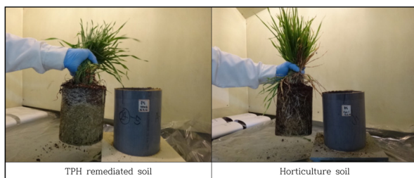
Fig. 3. Comparison of root development of rye after 38 days of cultivation in TPH remediated soil and horticulture soil.
