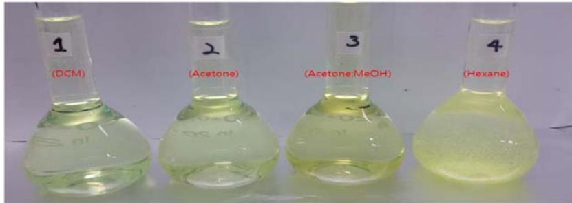
Fig. 2. Photograph on dissolution of high purity reagent BaP by different solvents used for preparing BaP standard stock solution.
