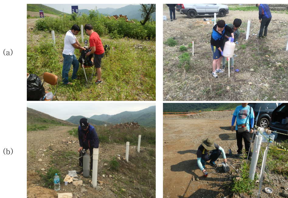
Fig. 3. Photographs of field activity. (a) Bio-regenerated iron mineral catalyst injection, (b) Ground water sampling and measurement.
