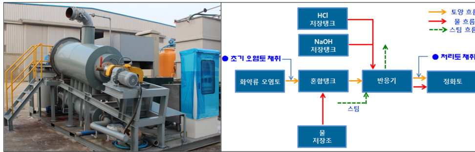
Fig. 4. Pilot scale experiment equipment for alkaline hydrolysis of explosives using in this study (Left) and the schematic diagram of process flow (Right).
