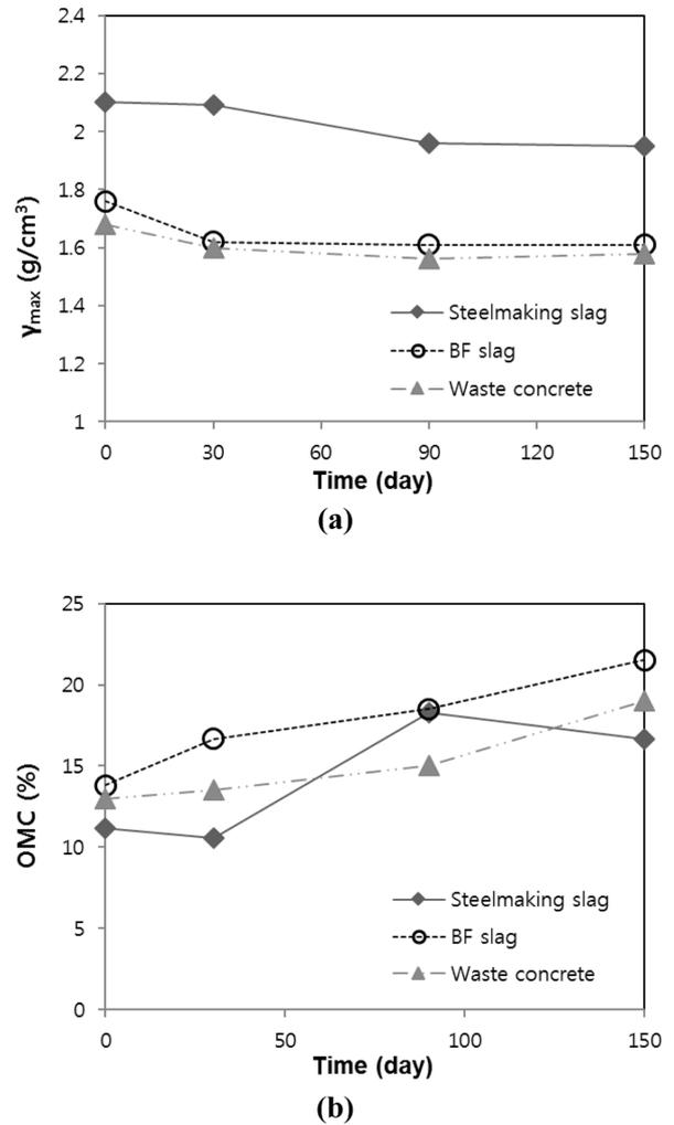
Fig. 4. Variation of compaction characteristics of (a) Maximum dry unit weight ( $\gamma_{max}$ ) and (b) Optimum moisture content (OMC) with aging period.
