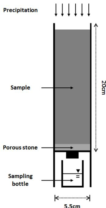
**Fig. 2.** A schematic diagram of test column.
