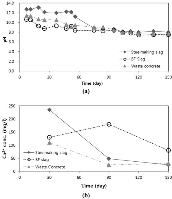
Fig. 3. Variation of (a) pH and (b) Ca<sup>2+</sup> concentration with time.
