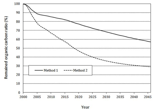
**Fig. 4.** Long-term estimation on the ratio of remained organic carbon in 2<sup>nd</sup> Landfill Site by Method 1 and Method 2 from 2001 to 2046.
