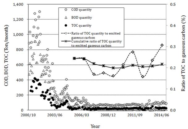
**Fig. 3.** Effluent quantity of organic carbon through leachate and its ratio to gaseous carbon emitted (2005–2014).
