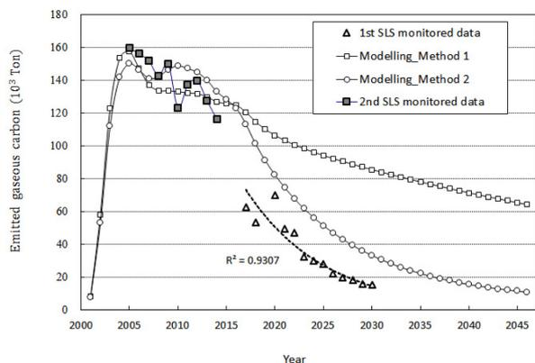
**Fig. 5.** The comparison of modeling results of 2<sup>nd</sup> SLS (by Method 1 and Method 2) to the post-closure monitored data of 1<sup>st</sup> SLS.
