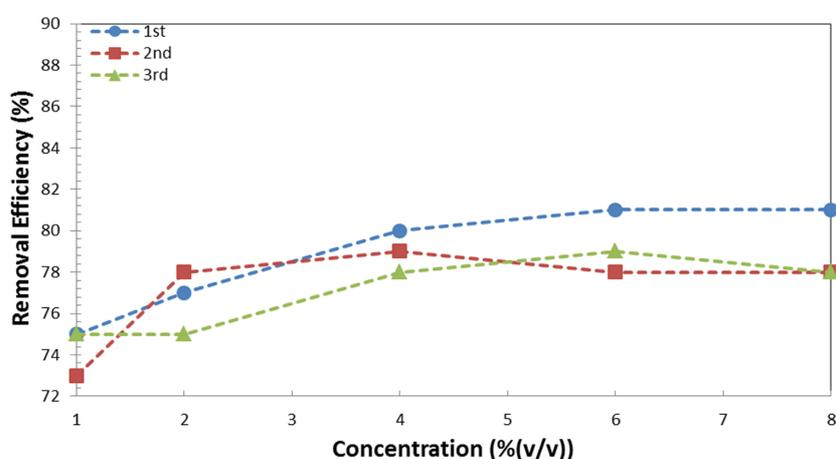
**Fig. 2.** The effect of surfactant solution concentration in SESF pilot tests.
