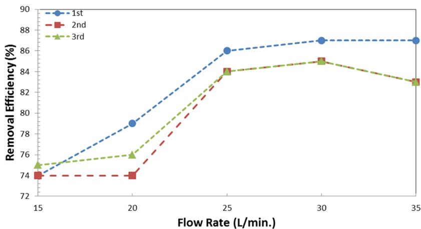
Fig. 4. The effect of surfactant solution flow rate in SESF pilot tests.
