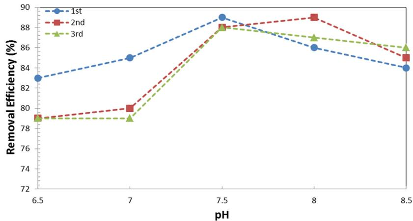
Fig. 3. The effect of surfactant solution pH value in SESF pilot tests.
