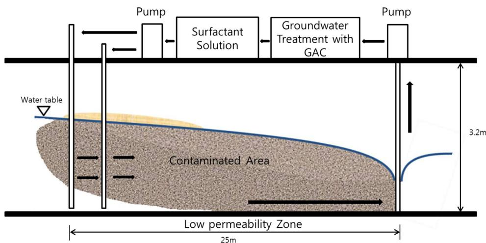
**Fig. 1.** The schematic diagram of surfactant-enhanced soil flushing (SESF) system at the demonstration site.
