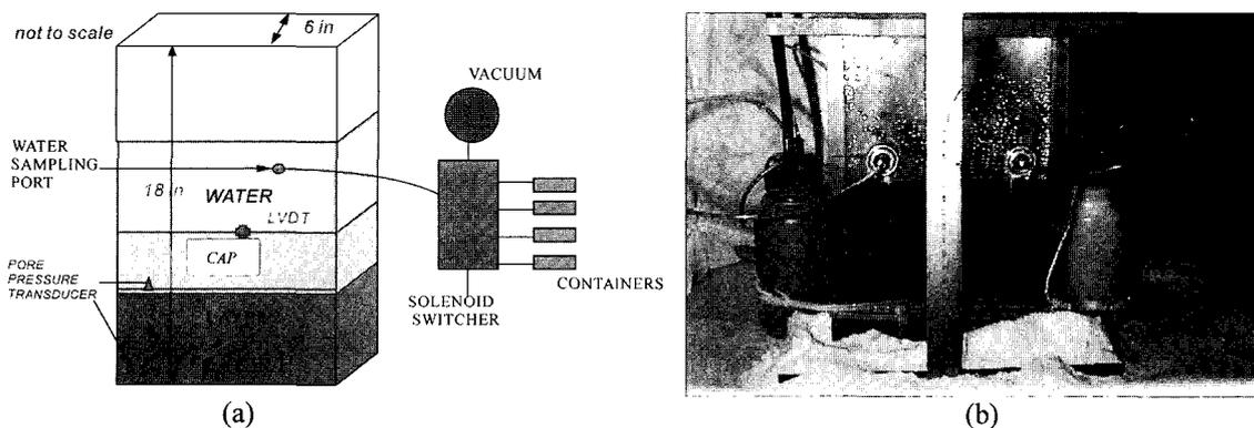
Fig. 3. (a) Schematic diagram of modeling box. (b) Environmental modeling box with sediment, cap layer and LVDT's.
