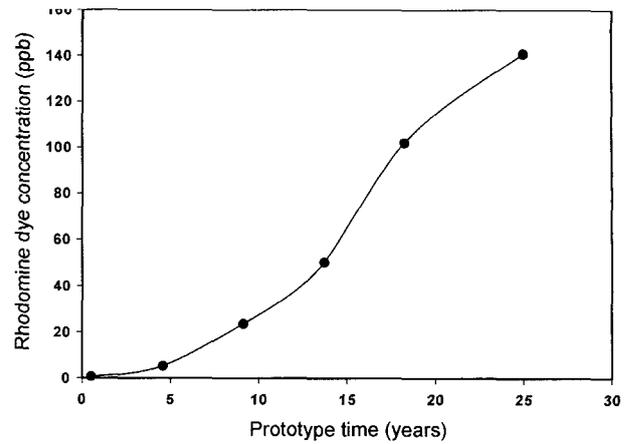
Fig. 6. Rhodamine dye concentration in advected pore water (centrifuge test I).
