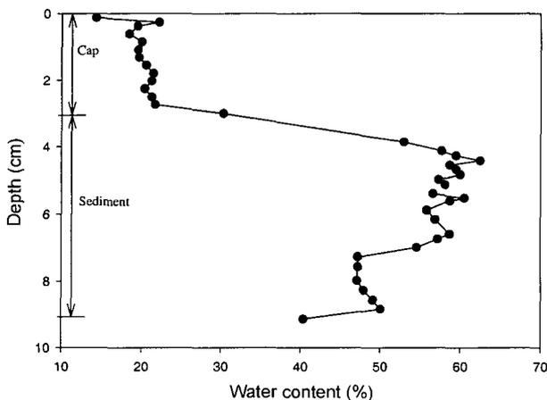
Fig. 5. Water content profile for the sediment and cap (centrifuge test I).
