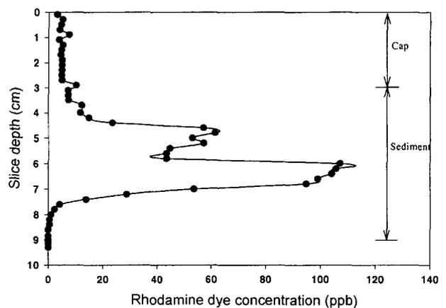
Fig. 7. Rhodamine dye concentration in sediment and cap (centrifuge test I).
