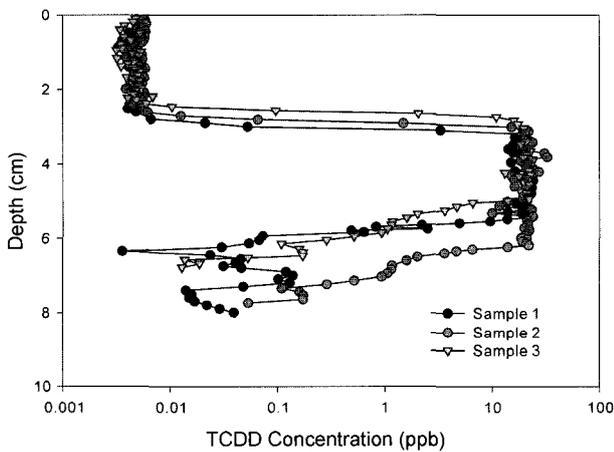
Fig. 9. TCDD concentration in sediment and cap (centrifuge test II).
