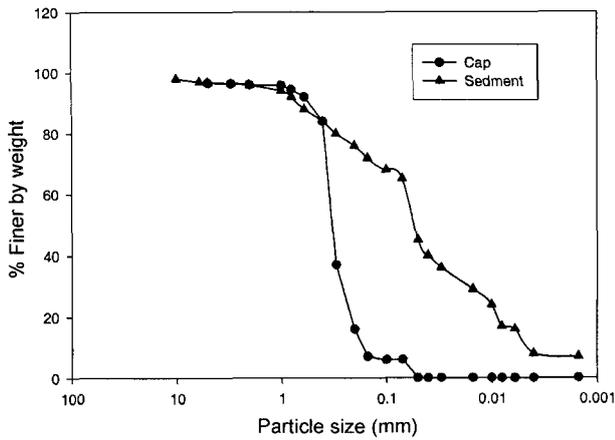
Fig. 1. Grain size distribution curve for sediment and cap.
