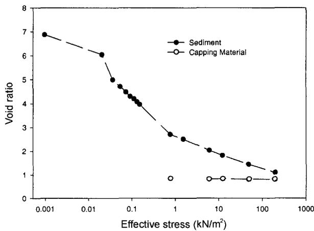
Fig. 2. Consolidation curve for NYDMMP sediment and capping material.
