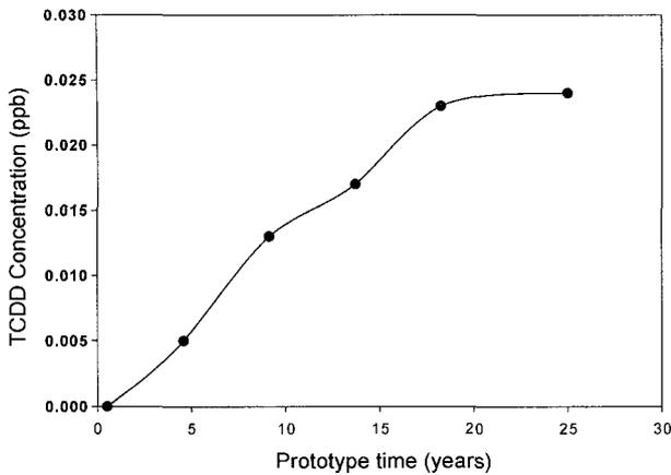
Fig. 8. TCDD concentration in overlying water (centrifuge test II).
