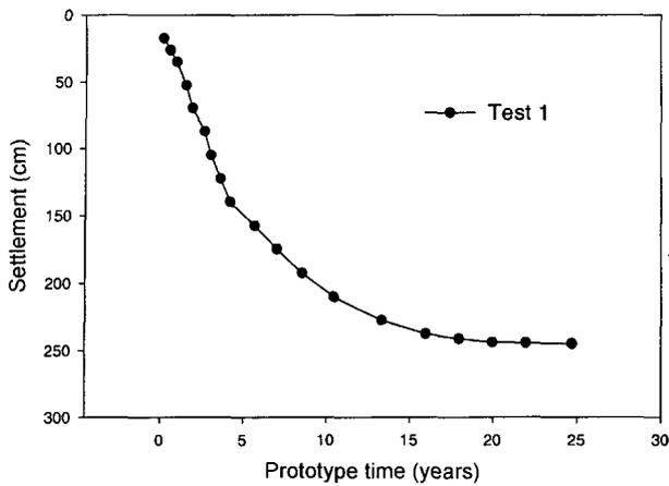
Fig. 4. Prototype settlement curve (centrifuge test I).
