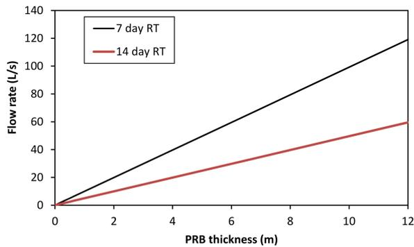
**Fig. 3.** Flow capacity for PRBs as a function of thickness, assuming residence time (RT) of 7 days and 14 days. A 1000 m width and 15 m depth of the barrier and an active pore volume of 40% were assumed.
