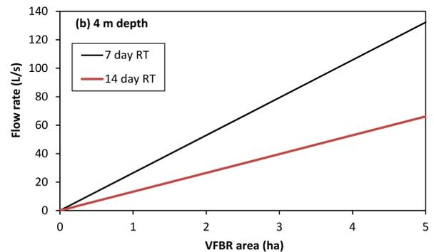
**Fig. 4.** Flow capacity for VFBRs as a function of surface area, assuming residence time (RT) of 7 days and 14 days. A (a) 2 m and (b) 4 m depth of the active vertical flow bed and an active pore volume of 40% were assumed. Note the difference in scale for the VFBR area between (a) and (b).
