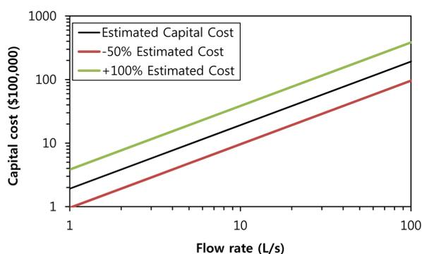
**Fig. 6.** Estimated capital cost for VFBRs as a function of flow rate.
