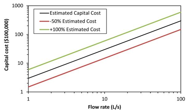
Fig. 5. Estimated capital cost for PRBs as a function of flow rate.
