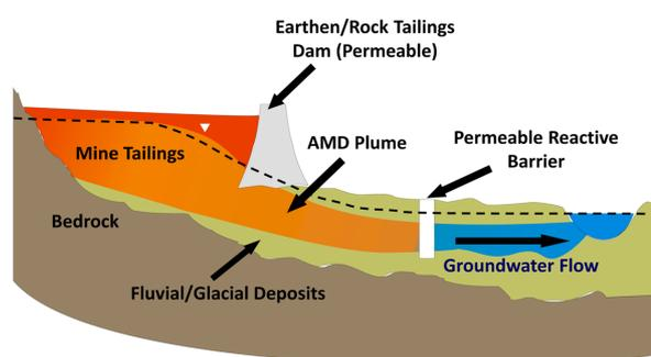
**Fig. 1.** Schematic of a PRB. Note that AMD represents acid mine drainage.
