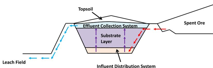
Fig. 2. Schematic cross section of a VFBR.
