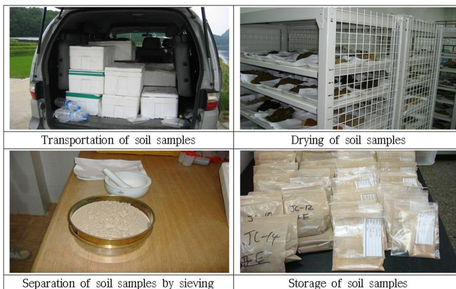
Fig. 1. The treatment of dredged soil samples in this study.
