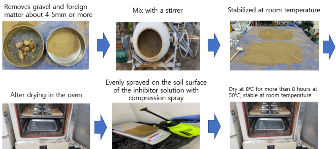
Fig. 1. Preparation of soil samples for wind tunnel tests.
