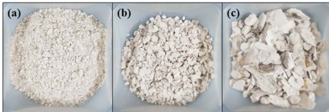
Fig. 2. Pyrolyzed oyster shells with different particle size (a:0-1 mm, b:1-2 mm, c:2-5 mm).
