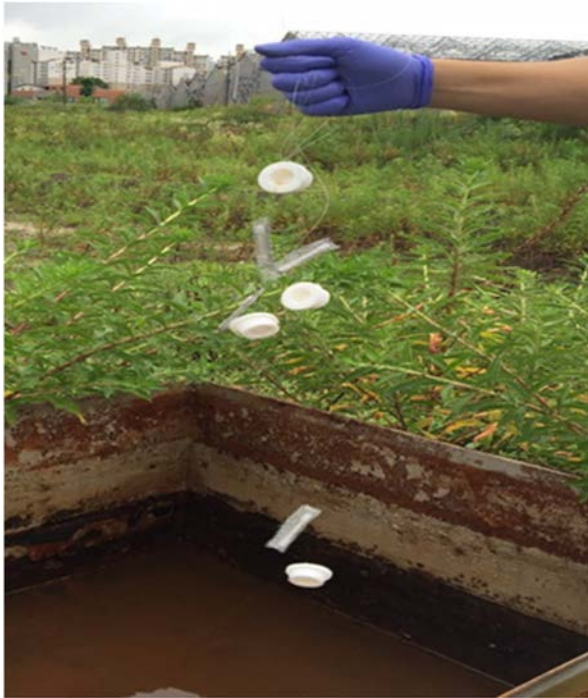
Fig. 3. Deployment of passive samplers to groundwater monitoring well.
