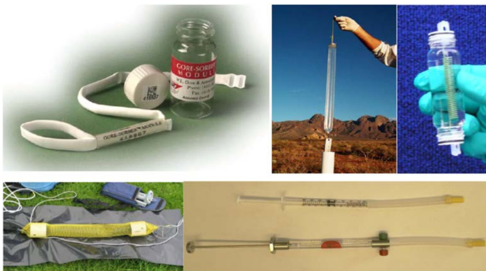
Fig. 4. Various types of passive sampler for VOCs (by turns, Gore Module, Hydrasleeve, Snap sampler, regenerated cellulose dialysis membrane sampler (ITRC, 2007b), syringe-silicone tubing samplers (Spalding and Watson, 2006)).
